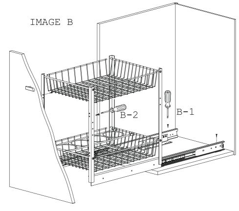
2-Fix to mechanism front zero to center of cabinet (IMAGE B).
